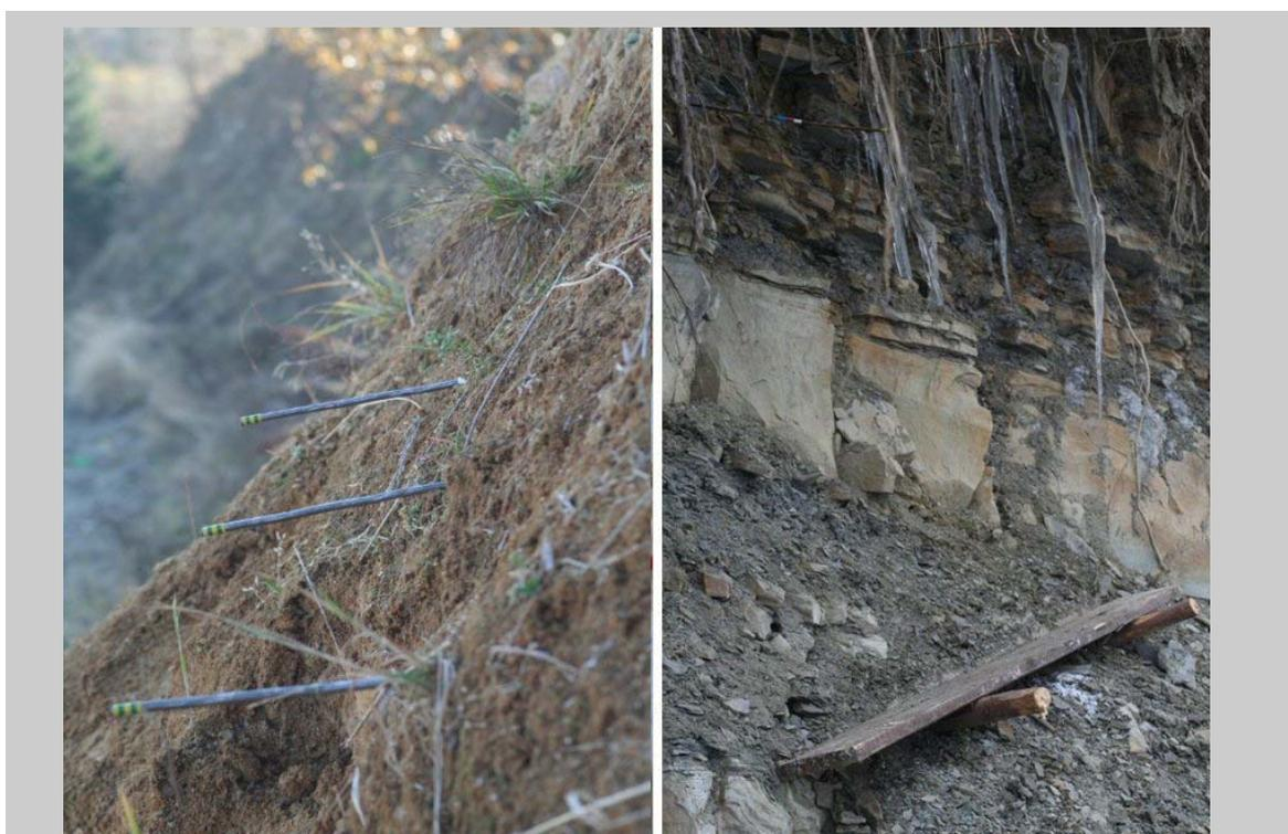
**Fig. 2** Erosion pins at site 1 (A) and bank sediment traps at site 3 (B)
