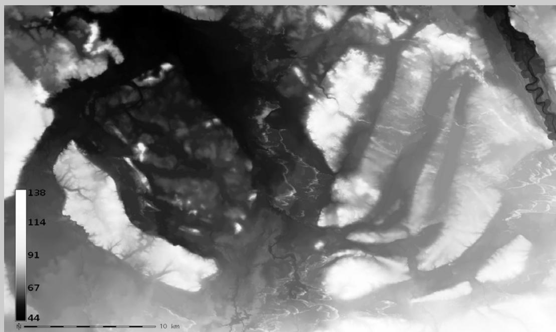
**Fig. 1.** Digital elevation model was done on the basis of 25 sheets of hypsometric map in scale of 1:10 000
